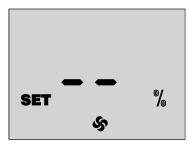
Access to the Fan Capacity Adjustment mode is confirmed by the **SET** and **%** indicators on the control panel display.
